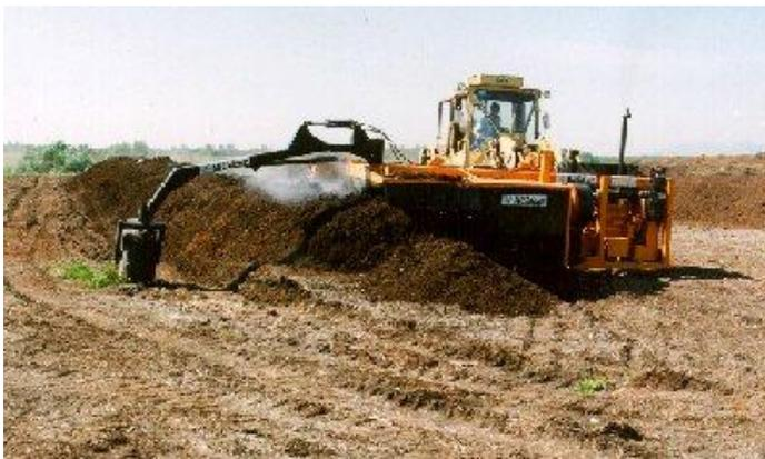
**Figure 2.2 Turning waste using Wildcat windrow turner**
